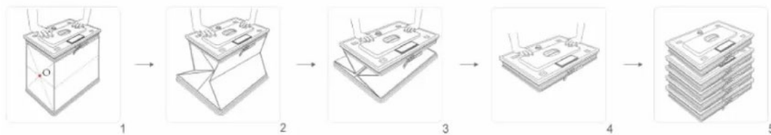
Figure 1 Schematic diagram of axial center type shear hinge folding structure
